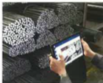
棒端端面計数機(手動式) Bar end surface counting machine (manual operation)
